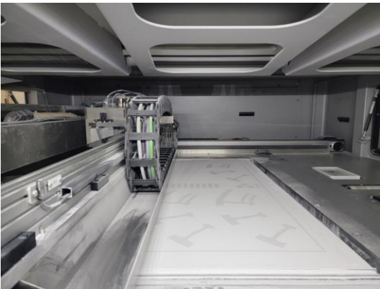
Image 2 - The VX1000 holds a build volume of 1000 x 600 x 500 mm
