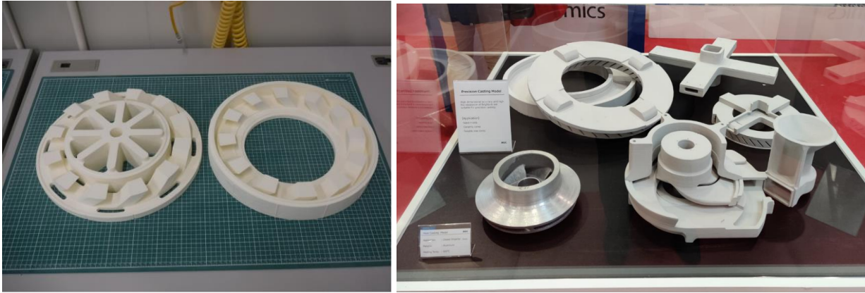
Image 3 – Investment casting cores 3D printed with Brightorb offer unique advantages in terms of chemical stability, heat resistance, thermal conductivity and low thermal expansion
